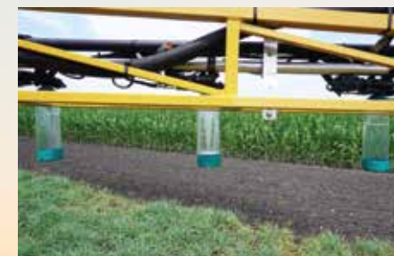
This nozzle had 75% blockage.
