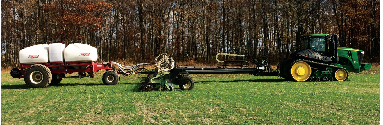
STICKING TO STRIP-TILL. While Mike Shuter strives to maintain as close to a no-till system as possible on his organic acres, he still finds it necessary to strip-till fertilizer ahead of his organic corn. He uses this 24-row Misenhelder Welding toolbar with Orthman 1tRIPr row units and a Salford fertilizer air cart. He uses a pelletized poultry litter in addition to the nutrients supplied by his cover crops.
