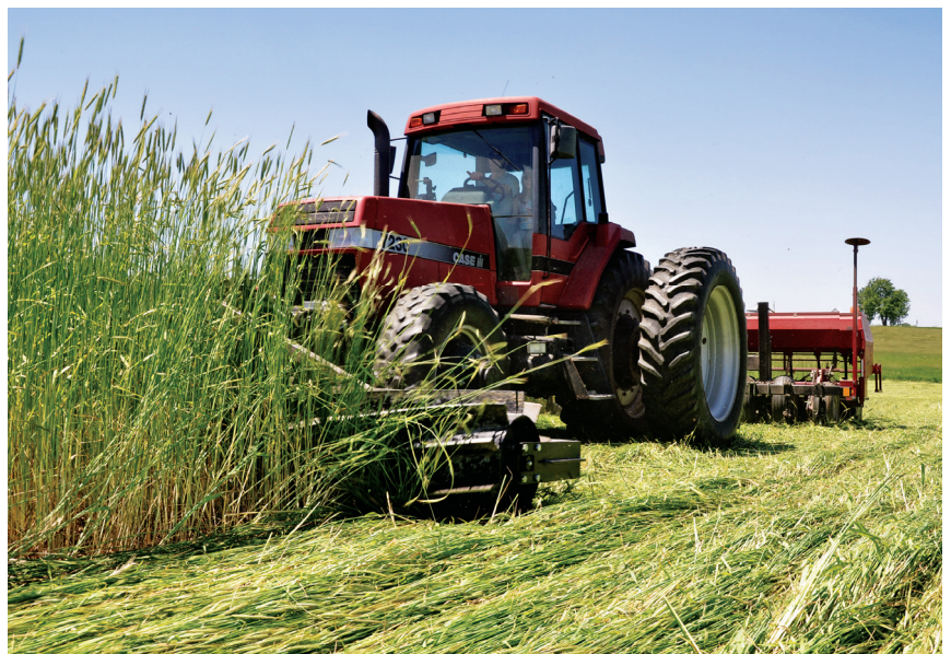
DOUBLE UP. A lighter roller-crimper allows Levi to mount it to the front of his tractor for one-pass cereal rye termination and soybean planting.
