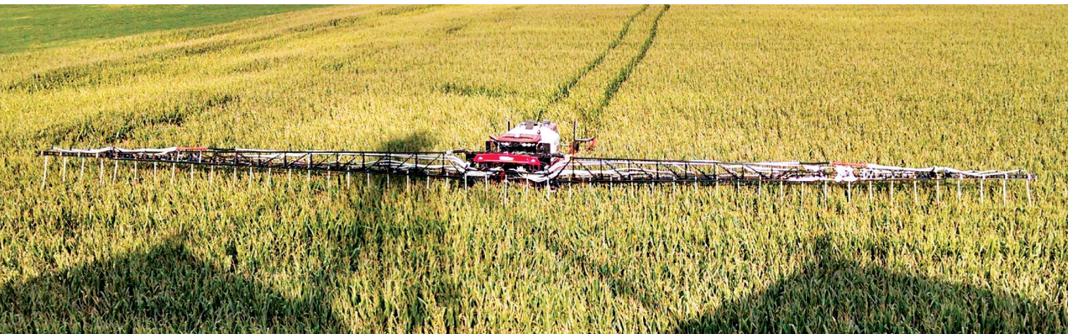
ADAPT, OVERCOME. The Shutters have a knack for engineering their way around a tough challenge. They’ve adapted their Miller Nitro sprayer to broadcast cover crops into standing crops (seen here) and reworked it into a water weeder to provide weed control in organic crops.
