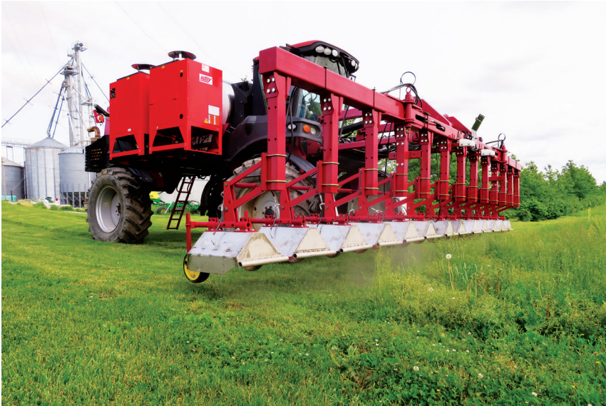
WATER WEEDER. The Shutters wanted a weed control option that would be safe for their soil life. Unlike fire or electricity weed control tools, or tillage, this custom-built machine kills weeds by scalding them with super-hot water.
